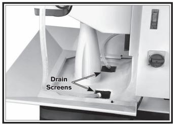
Figure 56. Locations of the coolant drain screens.
